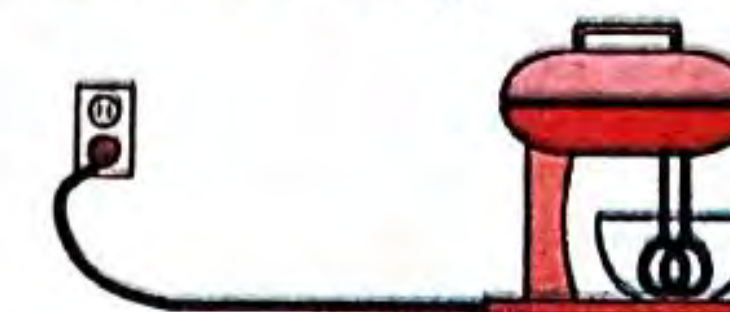
Figure 8.13 An electric mixer changes electrical energy to mechanical and heat energy.
