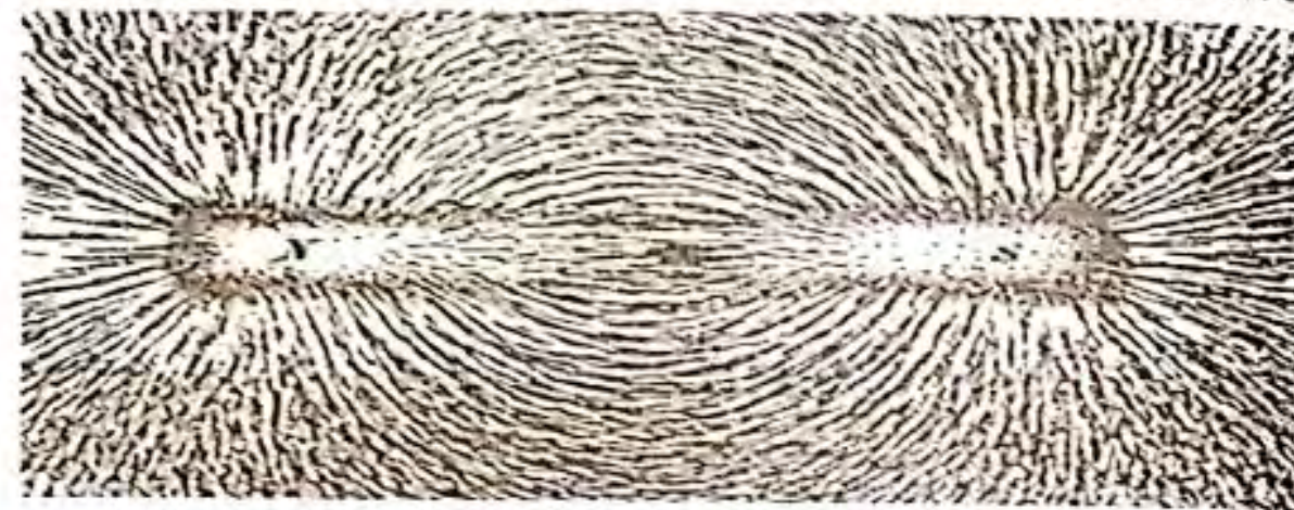
Figure 10.1 Magnetic field of a bar magnet
