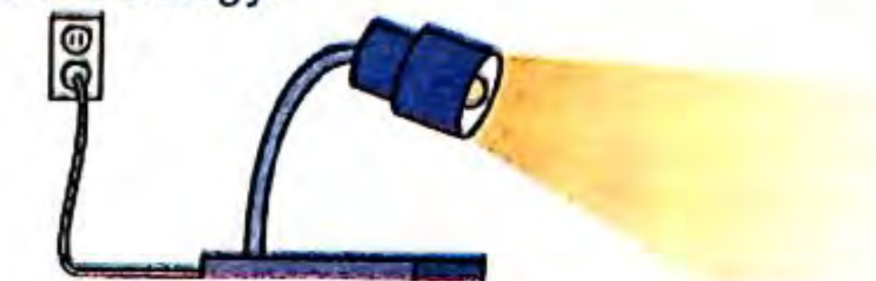
Figure 8.15 A lamp changes electrical energy to light and heat energy.
