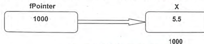
Figure 7.1: Use of the Pointer Variable
