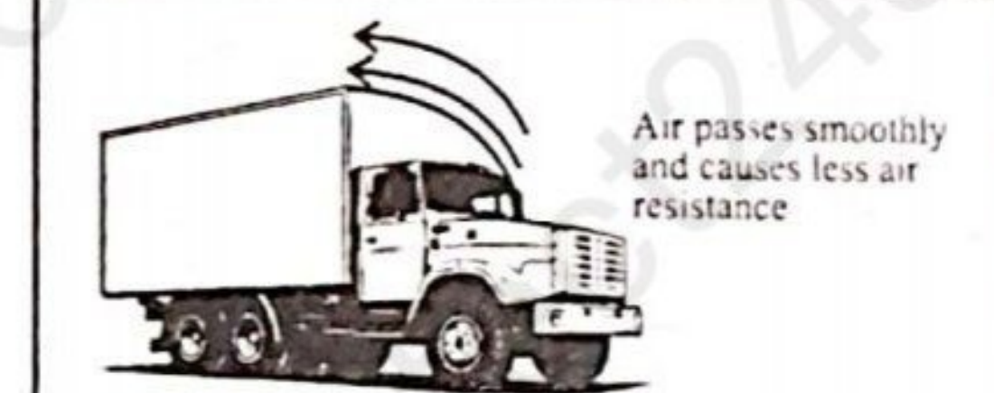
Fig b: Truck with wind deflector on top of their cab
