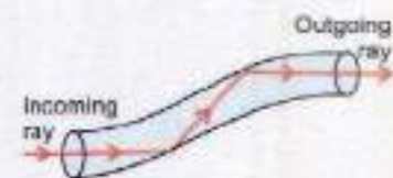
Fig. 10.10 (b) Light propagation within a flexible glass fibre.
