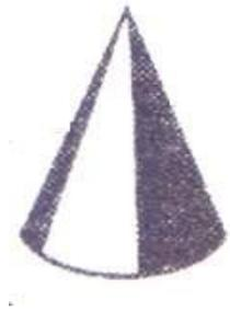
The Centre of gravity of the cone is nearer the base. When this cone is displaced, its Centre of gravity is raised. A cone in stable equilibrium should have its Centre of gravity as low as possible. The vertical line through its Centre of gravity should be within its base when the cone is disturbed. If the vertical line through the Centre of gravity is within the base, a torque due to weight of the cone brings it back to the original position.
